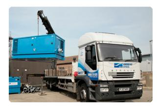
Performance Max head 105 m Max flow: 90 l/s Max solid 20 mm Weight 2905 kg Dimensions 4090 x 1370 x 1685 mm Noise Level @7m = 70 dBA
