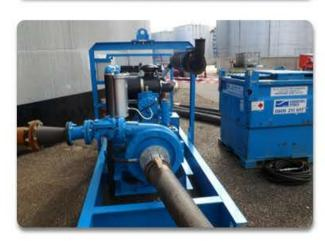
Weight 2100 kg Dimensions 4090 x 1370 x 1685 Performance Max head: 105 M, Max flow: 90 l/s, Max solid: 20 mm Fuel consumption Full load @ 1800 rpm: 26.5 litres/hour Pipe connections Suction: 6" Table D. Discharge: 4" NP16. Bauer
